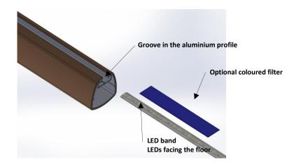
• If the profile is longer than one LED band, the bands must be connected to each other. To do this, use the single connector and the wire connector (peel the band adhesive on **1 cm** to facilitate the connection).
