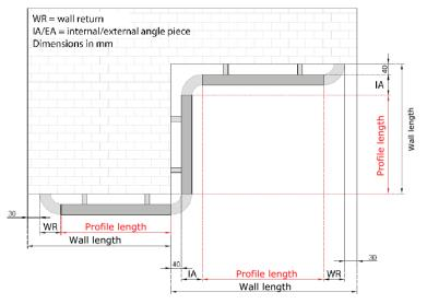
Based on the measurement of the wall minus the necessary clearance of 30 mm at the end(s), use the following table to calculate the lengths of the aluminium and PVC profiles to be cut depending on the accessories used:
