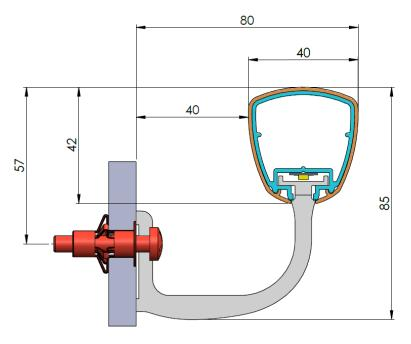
For a handrail height of 900 mm (measured at the handrail's upper surface), the drilling height is 843 mm (900 - 57).
