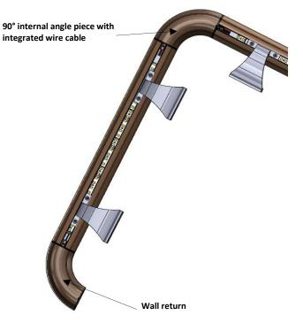
Finally, fix the brackets and wall returns to the aluminium profile using the 2 mm and 2.5 mm Allen keys.
