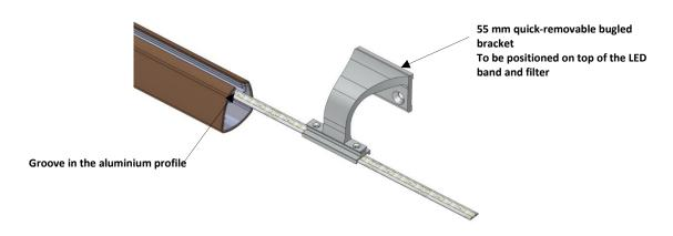
• Position the end brackets a maximum of 50 mm from the end of the profile.
