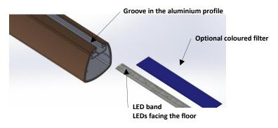
If the profile is longer than one LED band, the tapes must be connected to each other. To do this, use the single connector and the wire connector.
