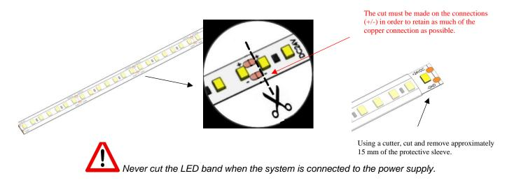
• Connect the wire connector (driver side) to the LED band.
