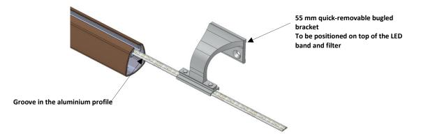
• Position the end brackets a maximum of 50 mm from the end of the profile.
