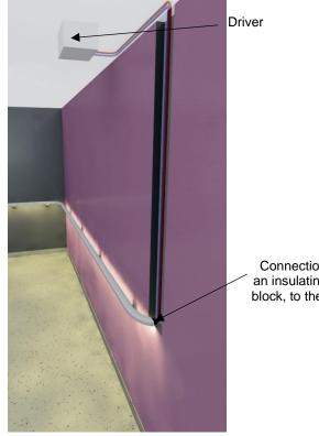
Connection of the handrail, using an insulating screw joint or terminal block, to the power cable at the wall return
