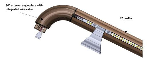
Position and assemble the wall return at the power supply side (pass the wire connector through the hole provided).
