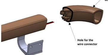
Connect the wire connector of the angle to the LED band of the 2nd profil (peel the band adhesive on 1 cm to facilitate the connection) respecting : connect the red wire to the positive terminal and the black wire to the negative terminal of the LED band.
